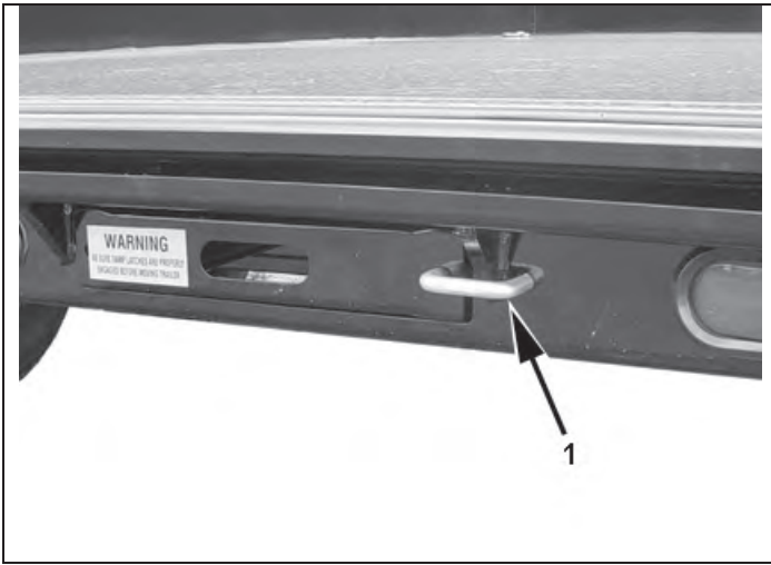
Figure 5-4 - Lock Ramps With Pins
