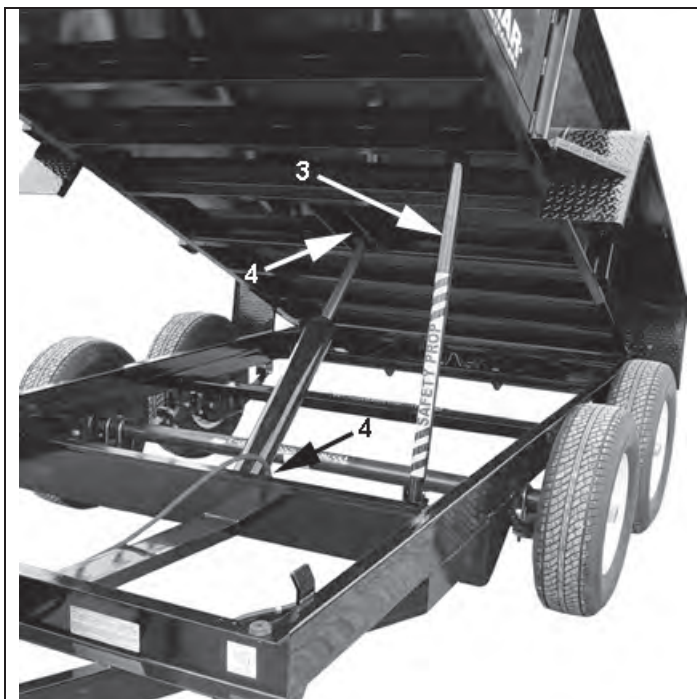
Figure 8-3 - Support Body and Lubricate Cylinder Ends
